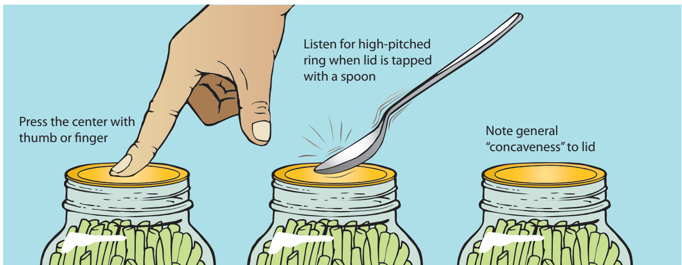
Figure 8. Testing the seal.
